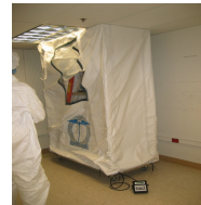
Environmental containment unit (ECU)
