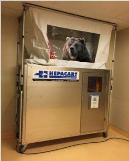
Environmental containment unit (ECU)
