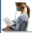
A fit test is conducted to verify that a respirator is both comfortable and correctly fits the user. Fit test methods are classified as either qualitative or quantitative. A qualitative fit test is a pass/fail test that relies on the individual's sensory detection of a test agent, such as taste, smell, or involuntary cough (a reaction to irritant smoke\*). A quantitative fit test uses an instrument to numerically measure the effectiveness of the respirator.
